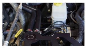
The contents of the catch can should be checked and drained every 1000 miles until a baseline for oil accumulation is established. The volume collected in the can will be different for every car and will vary based on climate, temperature, and driving conditions.
