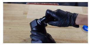
6. Install the catch can to the bracket using the hardware included with your kit. (3x 2.5mm screws and washers)
