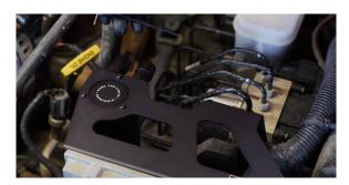
7. Disconnect the ignition coil electrical harness to gain better access to the spring clamp at the PCV valve. To do this, lift the red tab on the harness and then depress the gray tab at the center.
