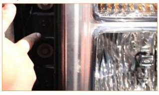
**5.** Remove the lower grille bracket. Remove 1x pop clip, 4x 13mm bolts (two on each side), and 2x 10mm bolts (one on each side). Unclip the bracket by pulling outward on the tabs located on the upper part of the mount.
