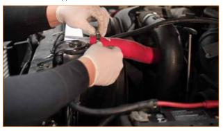
14. Reinstall the air box and intake hose.
