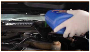
**20.** Start the vehicle and set the heat on high. Allow the vehicle to reach operating temperature so that any air from the cooling system will be purged. Be sure to inspect the cooling system for any leaks.
