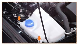
02. Release the AC line from the plastic clip on the side of the washer tank.
