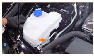
03. Lift the washer tank up a few inches to access the electrical harness on the bottom of the tank. Separate the brown connector from the fluid level sensor by depressing the tab and pulling the connector out of the sensor.
