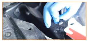
6. Disconnect the grille shutter, camera, and washer fluid harnesses. These can be found in front of the hood latch connector.
