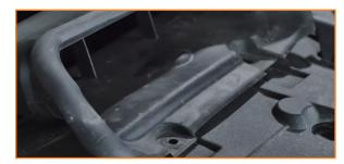
Release the clips that secure the corner panels. (2x pop-clips)
