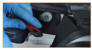
Release the clips that secure the radiator cover and remove it. (8x pop-clips)
