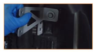
16. Install the transmission cooler to the brackets. The transmission cooler can be installed in two orientations. For the F-150 2.7L & 3.5L EcoBoost, install the cooler with the inlet & outlet facing up, and relocate the tree clip on the hose to the riveted bracket on the bottom.
