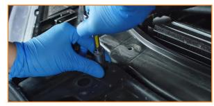
9. Remove the bolts at the bottom of the grille.
