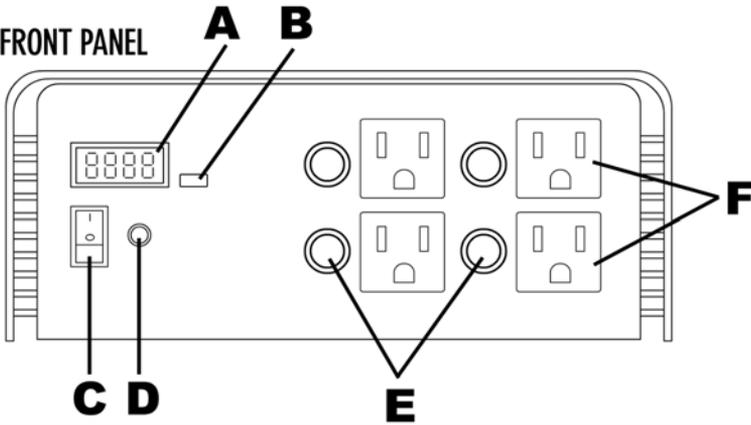
**A.** Digital Display for DC Volts or AC Watts.
