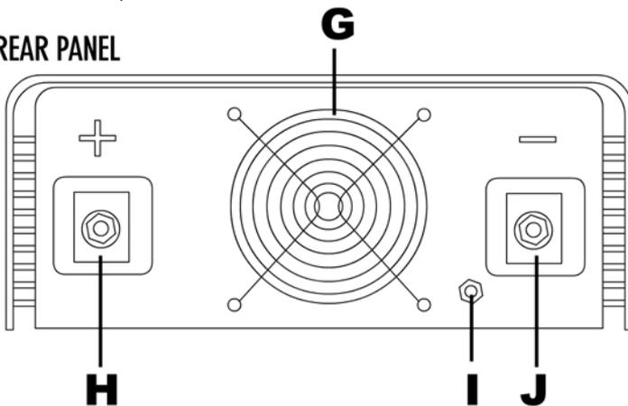
**G.** High-Speed Cooling Fans. When the temperature inside the inverter exceeds a preset limit, the Cooling Fan automatically turns on to cool the inverter. When the temperature reduces, the fan turns off.
