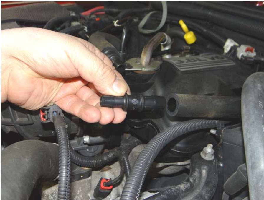
Step 6: Insert 1/2"x5/8" coupling into PCV hose.
