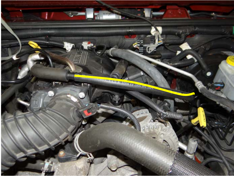
Step 7: Insert 12" length hose over coupling as shown.
