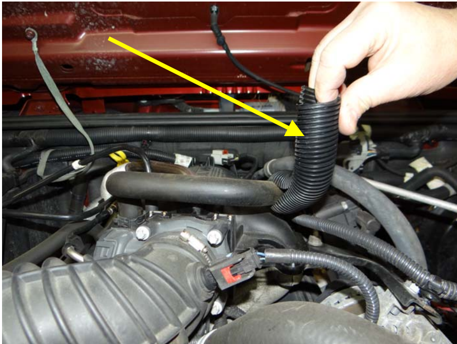
Step 2: Remove outer jacket as shown.
