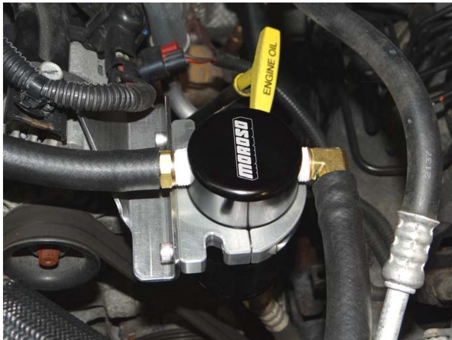
Step 16: Connect hoses to air oil separator.
