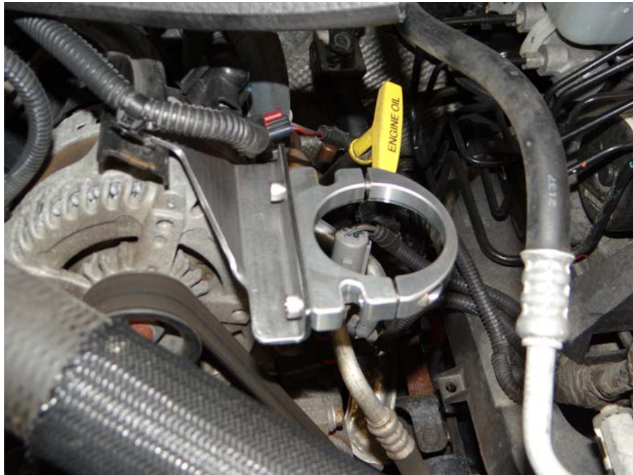
Step 12: Assemble billet clamp assembly to stainless mounting bracket using (2) 1/4-20x5/8 SHCS. Reliefs must face down.
