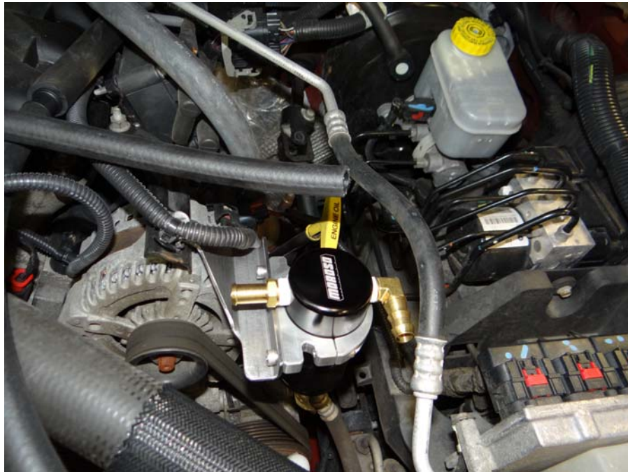
Step 14: Insert into billet clamp.
