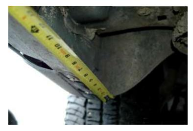
Measure from front wheel well back Std Cab— 16" & 48" Super Cab—17", 33 1/2", 64" Super Crew Cab—17", 47", 70"
