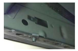
Pull the tape that covers large hole in rear of rocker panel. Slide a spring clip into hole until it snaps into the other hole.
