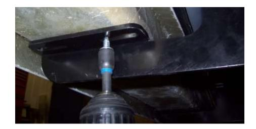
Place the board on the brackets and align up on the vehicle. Attach to the brackets using  $\#14 \ge 3/4$ " long self drilling screws.
