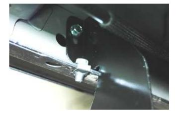
Attach brackets to vehicle by inserting a 5/16" x 3/4" bolt into the spring clip and 5/16" x 3/4" bolt and nut through the pinch weld hole.
