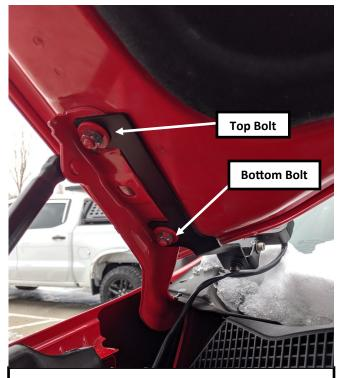
Figure 2: Bracket Installation.
