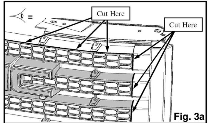
12. Carefully cut out the center section of the factory grille. Use the dashed lines in figure 3b as a guide for cutting. When you have removed the center grille section it should look like figure 3c.
