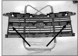
Remove (2) 7mm bolts (locations shown above)from back of grille. Unclip chrome tabs and bowtie tabs (use flat head screw driver). take bowtie and middle chrome section of grille off.
