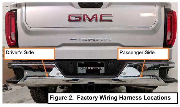
1. Factory wire harness are located behind the rear bumper, near the spare tire, frame rails, and exhaust. Shown in Figures 2 and 3.
