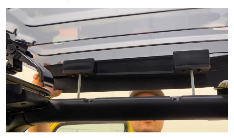
**Caution:** Leave the RED bolt covers on while installing the Sky View to avoid scratching paint while installing the Sky View lid.
