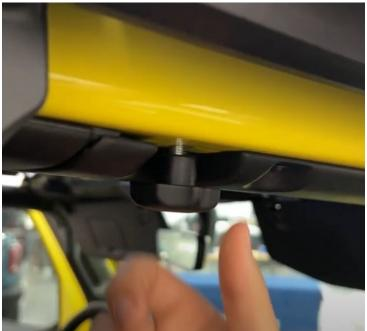
4. Tighten the M8 knobs leaving a small gap between the Sky View hardware and the roll bar on the vehicle. Do not overtighten.
