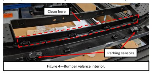
7. Remove the film from the double sided tape on the grill insert. To install the grill insert onto the bumper valance, line up the slots in the mounting tabs with the slots cut in the bumper for the license plate bolts. Push down on the grill insert so it follows the curvature of the bumper valance and slide it upwards until the tape contacts the underside of the lip. Squeeze together the bumper and tape tabs to make sure there is adequate contact of the tape. (**Figure 5 & 6**)
