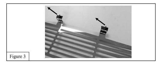
5. Tilt grille into bumper opening, bottom first, tabs on the top go behind upper bumper. On some trucks these tabs will go between a black bracket and the upper bumper, refer to Figure 4.
