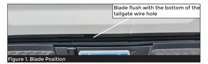
Remove tape release liner on all brackets. Place light bar in position on the bed of truck, insuring proper gap shown in (Figure 1). Do not stick tape to truck until light bar is in correct position. Light bar wire should exit toward driver side of truck.
