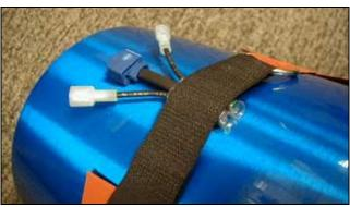
2. Secure the heater element around the bottle with the Velcro straps attached to the heater element.
