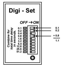
This time delay switch is set to activate a 2nd stage of nitrous after a delay of 1.1 seconds.
