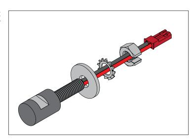
5. Connect LED License Plate Bolts to the spliced Male Connectors. Turn on lights and aim correctly at license plate.
