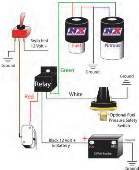
7. Attach the remaining wires from each of the solenoids to a ground. Note: These coils are direct current and it does not matter which wire is used.
