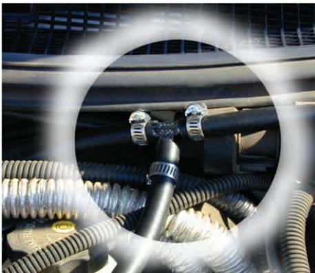
**WARNING: The fuel rail and/or fuel lines are under high pressure. Use extreme caution when disconnecting any fuel line. Quickly collect and properly dispose of any excess fuel spillage.**
