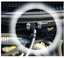
WARNING: The fuel rail and/or fuel lines are under high pressure. Use extreme caution when disconnecting any fuel line. Quickly collect and properly dispose of any excess fuel spillage.
