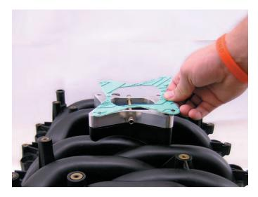
Next, using the supplied gasket, reinstall the upper intake elbow on the nitrous plate. Once again double check your nitrous and fuel configuration, making sure the plate has the word "TOP" up and "Fuel" is facing the front of the vehicle.
