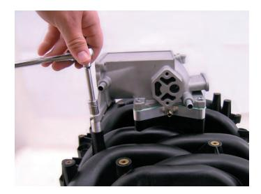
Now it is time to install the proper jets in the plate fittings. Make sure the number on the side of the jet corresponds with the proper number for the desired horsepower setting. You will repeat this process for the nitrous and fuel side of the plate.
