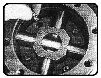
Figure 10 Install pinion shafts, block, pins and springs
