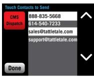
Phone numbers and emails input in the system will appear on screen. Touch to select contacts that will receive Hot Button alarm messages. Input additional contacts
