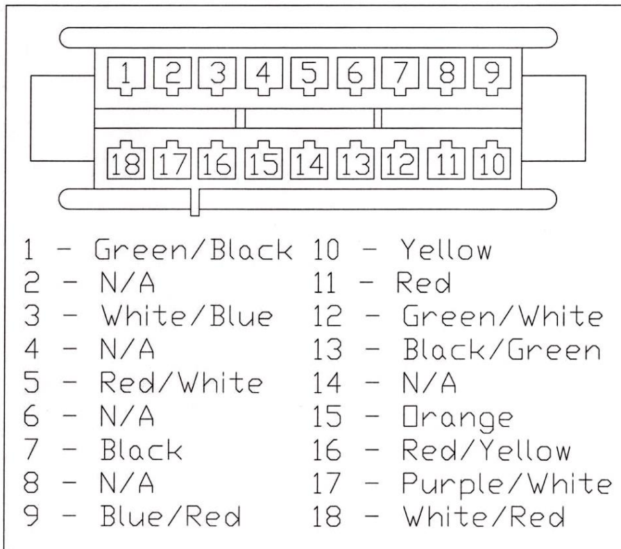
Figure 7-38 1973 - 1974 Cluster Pigtail Pinout
