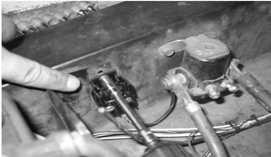
Figure 7-5 Installing the Maxi Fuse Holder '67-'72 Models
