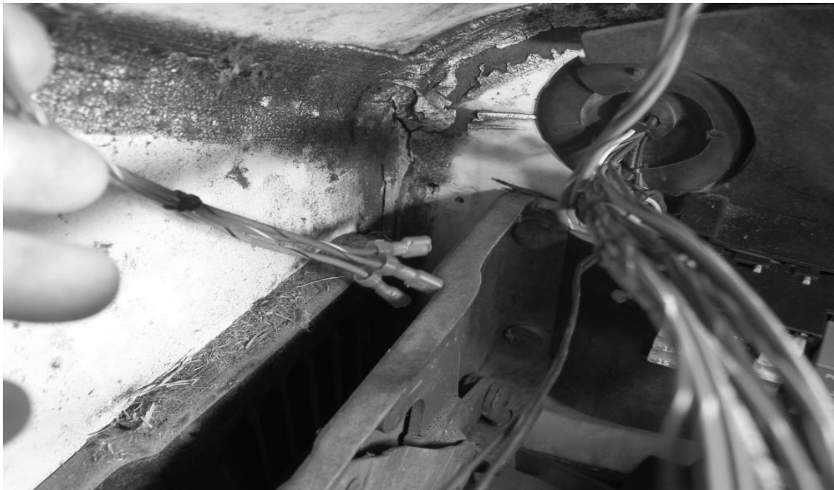
Figure 7-22 Routing the Dimmer Switch Wires
