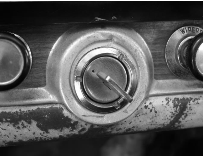
Step 1 – Turn Switch to ACC. POSITION
