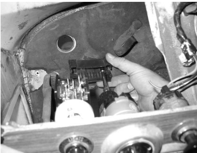
Figure 6-2 Fuse Block Base Position '67-'72
