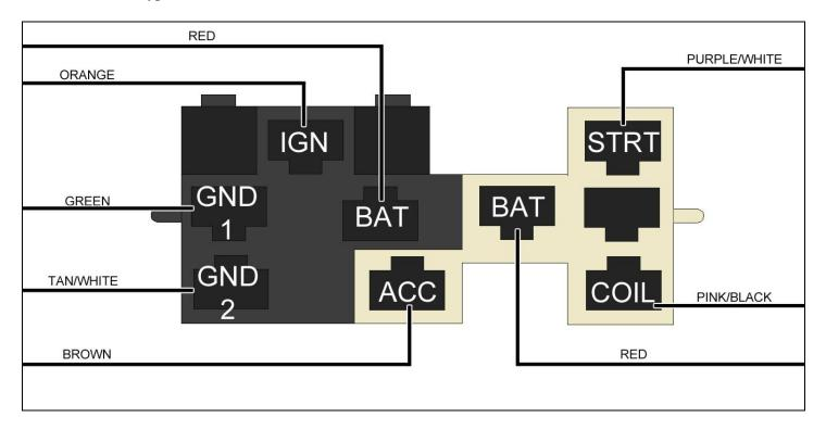
**IGN**: Switched power to fuse block, this pin will only have power when the key is in the ON/RUN position. This pin uses the larger/wider terminals.
