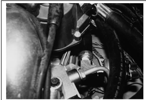
**Figure 10** Oil Pressure Switch
