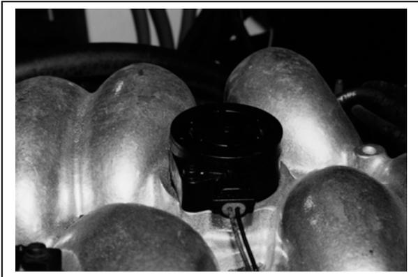
**Figure 9** Variable Tuning Control Solenoid (VTC)
