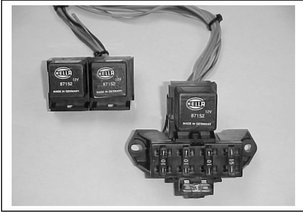
**Figure 1** Fuse Block, Fuel Pump Relay & VTC Relay
