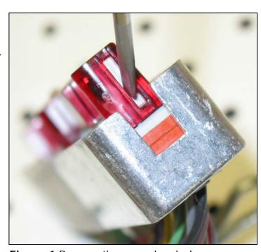
**Figure 1** Remove the secondary locks.
