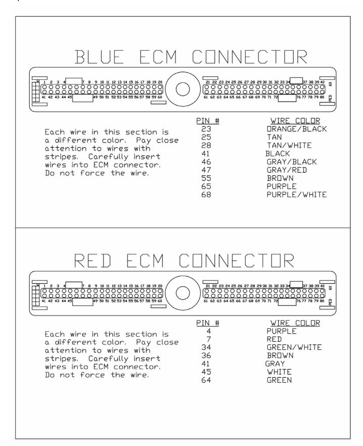
Figure 2 ECM connectors pin out
