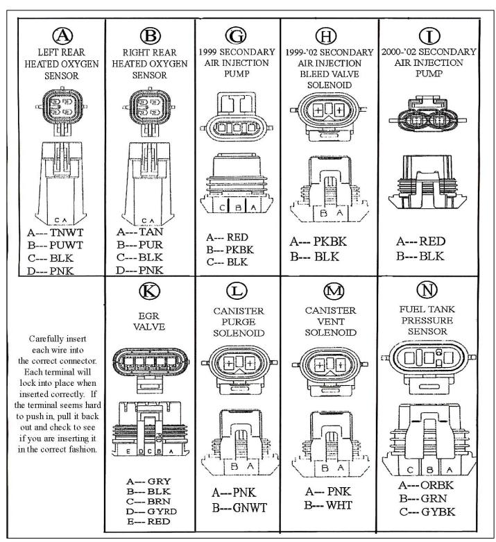
Figure 3 Emission connector pin out chart
