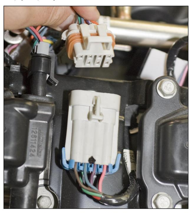
Route the throttle body connector over to the throttle body. Plug it in as shown below.
