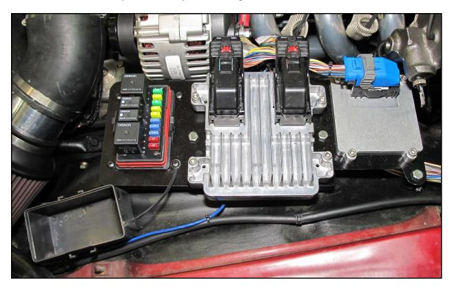
**NOTE:** Looking at the picture above you see how the connectors plug into the ECM and TCM. It is important that you leave room for these connectors when deciding on your mounting solution.
