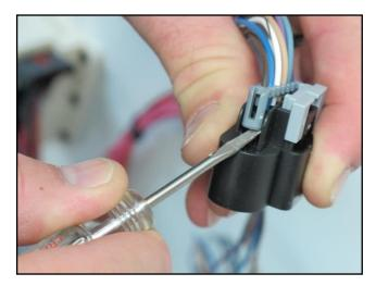
2. Remove the terminal position assurance from the connector.
