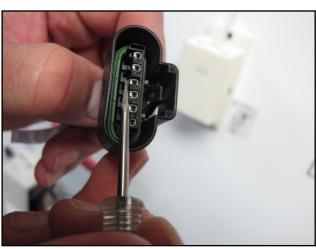
4. The connector pin out should now be how it is shown here. Reinstall the terminal position assurance and secondary lock to the connector.
