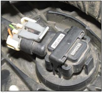
If you have the factory installed fresh air intake from the donor vehicle you should have then also gotten the mass air flow sensor. It should look something like what is shown below. Route the m.a.f. connector over to the m.a.f. sensor and plug it in.
