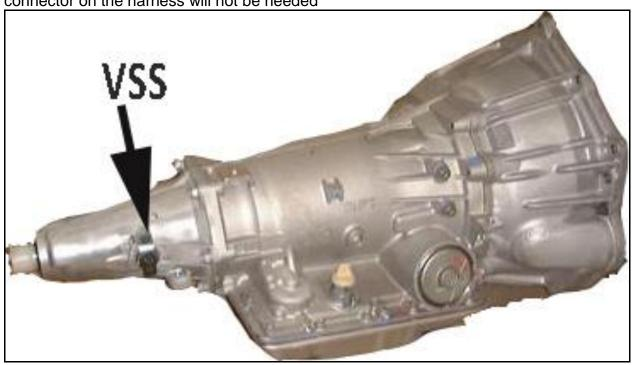
4L80E and 4L85E transmissions have a vehicle speed sensor and also an input speed sensor located on the driver side of the transmission. Below is a picture of a 4L80E transmission for reference.
