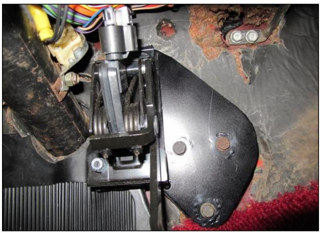
1. Remove the secondary lock from the connector.
