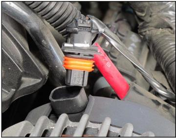
Route the cam position sensor connector down the front of the engine and over to the cam position sensor. If your engine has variable valve timing you will find this connector has five pins. The Painless harness has a pigtail plugged into the mating connector for this 5 pin connector. Unplug the pigtail and plug the Painless harness five pin connector into your cam position/cam phazer connector.
