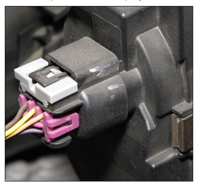
Route the m.a.p. sensor connector up to the m.a.p. sensor, which is located front and center top of the intake manifold. Plug it in as shown here.
