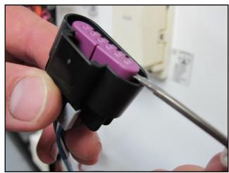
Switch wires in pin D and F with each other in the connector.
