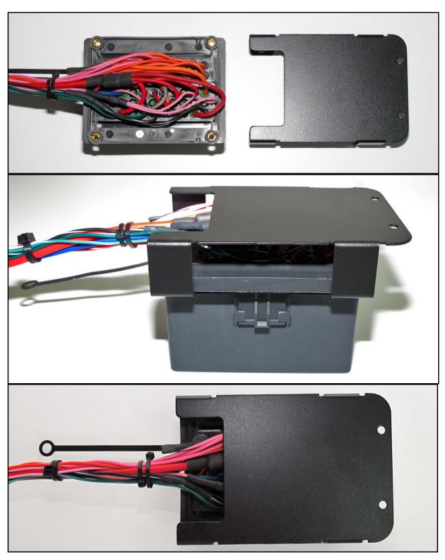
Use the four black machine screws to mount the fuse block to the fuse block mounting bracket. Then use your choice of mounting screws to secure the bracket to it intended mounting point in your vehicle. Most people use self tap screws or machine thread screws.
