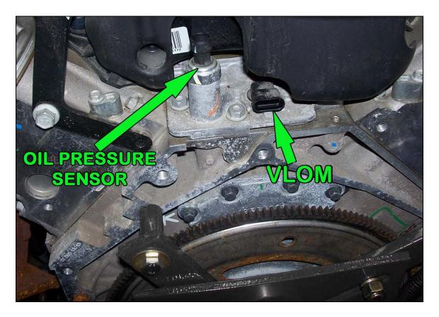
At the back of the motor is the oil pressure sensor, plug the connector into the sensor.
