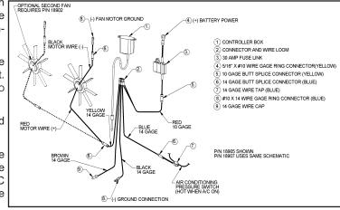
The BLACK wire in the loom is the ground wire. Attach this to the vehicle body or frame or other metal, grounded surface.
