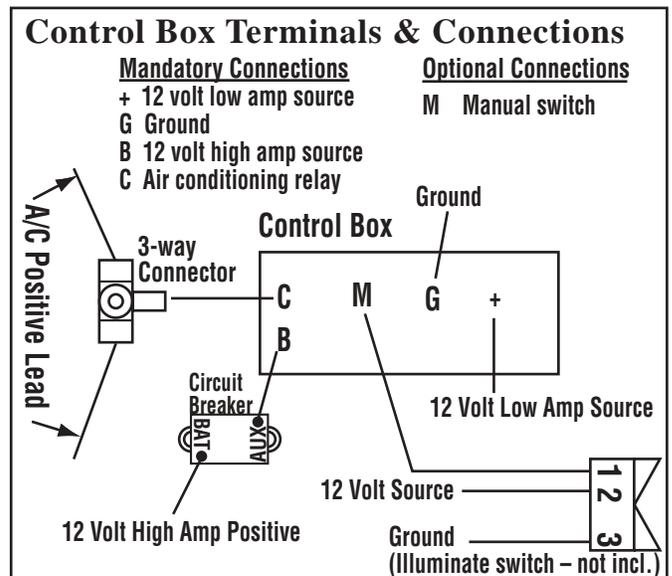
**IMPORTANT:** If not using an illuminated switch, disconnect the switch ground.
