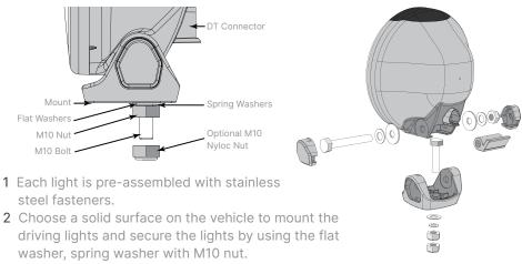
**3** An optional M10 Nyloc nut is included to provide extra security and vibration resistance.
