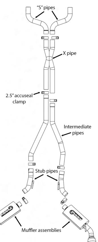
Tools Required: 15mm Socket Ratchet Spray lubricant
