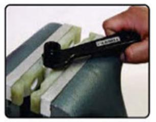
Step Four: Hold socket/hose in vise. Turn nipple with wrench until there is less than 1/16" between nipple hex & socket. Then, flush hose assembly w/solvent or soapy water and blow clean with compressed air or let air dry.
