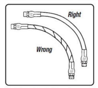
Avoid installing the hose in a twisted position.
