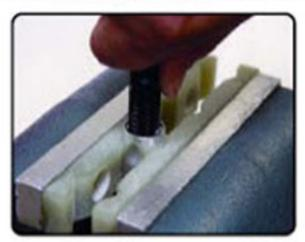
Step Two: Unscrew socket from hose end. Push hose into socket, turning counter-clockwise, until hose is seated against step in socket. Make sure rubber part of hose does not protrude into socket threads.
