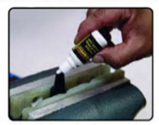
Step Three: Apply Russell assembly lube to threads on nipple assembly and in socket. Insert nipple into socket/hose and start threads by hand (clockwise).
