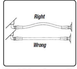
Allow slack in your hose assembly for changes in length that occur under pressure.
