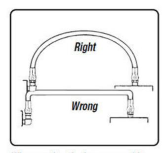
When routing the hose assembly, provide a smooth bend radius. Avoid sharp bends, which will collapse the hose I.D. and could restrict flow.
