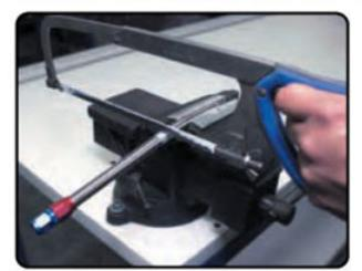
Step One: Wrap hose tightly with race or electrical tape at the point determined for cut. Clamp the hose loosely in a vise close to the tape. Use a hacksaw with two blades opposing one another or abrasive cut-off wheel. Remove the tape when you are finished cutting.
