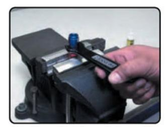
Step Four: Start the socket over the nipple by hand and tighten as far as possible by hand. Using an AN wrench, tighten until it reaches the nipple hex or when there is no more than 1/16" gap between the nipple/socket assembly. Be sure to wash & pressure test the assembly before using.
