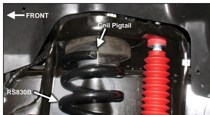
Driver side coil spring after rotating 90° from OE position
