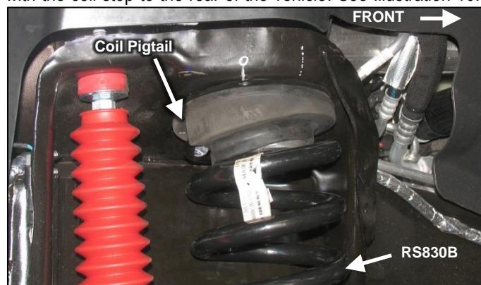
Passenger side coil spring after rotating 90° from OE position
