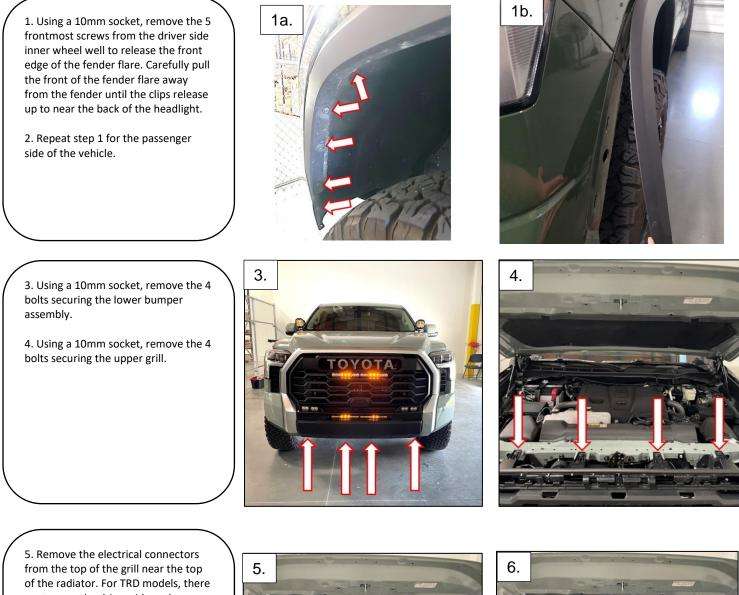
5. Remove the electrical connectors from the top of the grill near the top of the radiator. For TRD models, there are two on the driver side and two on the passenger side. For non-TRD models, there are two on the passenger side and one on the driver side.
