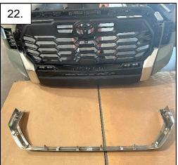
23. Locate and, using a trim tool, unclip the tabs securing the grill to the front clip.
