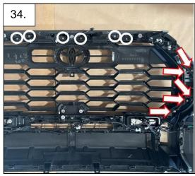
35. Using a 10mm socket, reinstall the shutter assembly using the 6 removed bolts (arrowed) and connect the shutter assembly harness (circled). Route the S8 power cord up to the upper passenger side of the grill towards the other wire connectors.
