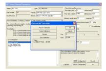
8. The status of the A/F channel will be displayed at the bottom of the dialog box. Before performing a calibration, make sure the sensor is not still warming up and that there are no errors. The Heater Calibration button is not used. If you have installed a new sensor in this channel perform a free air calibration. When you have finished click on the OK button to exit.
