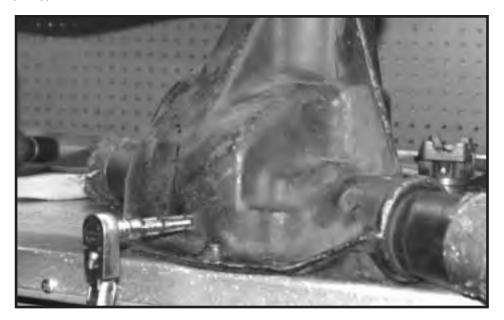
• Using a 1/4" NPT tap, tap the hole from the outside.
