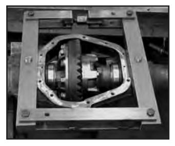
• Inspect housing to ensure there is proper oil drainage in both axle tubes. Failure to do so could result in damage to your Zip Locker<sup>™</sup> in addition to oil leakage from axle seals.
