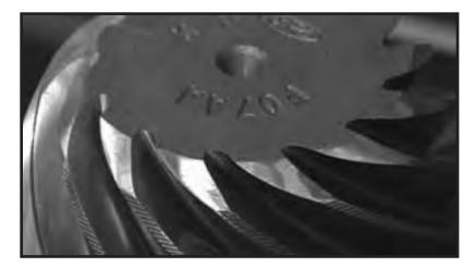
This modification of the pinion head will not affect its performance or strength. The area you will be removing is usually well outside the contact pattern.
