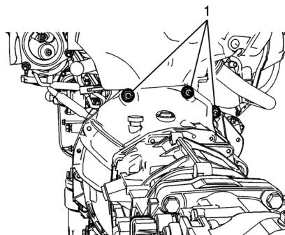
9. Fabricate and install the transmission mount. Mount is not included as this part will be unique to customer application. Part shown below for reference is from 2015 Cadillac ATS. Four bolts p/n 11562426 M10x1.0x30 mm are included for customer convenience. Torque is **58NM (43 lb ft)**.
