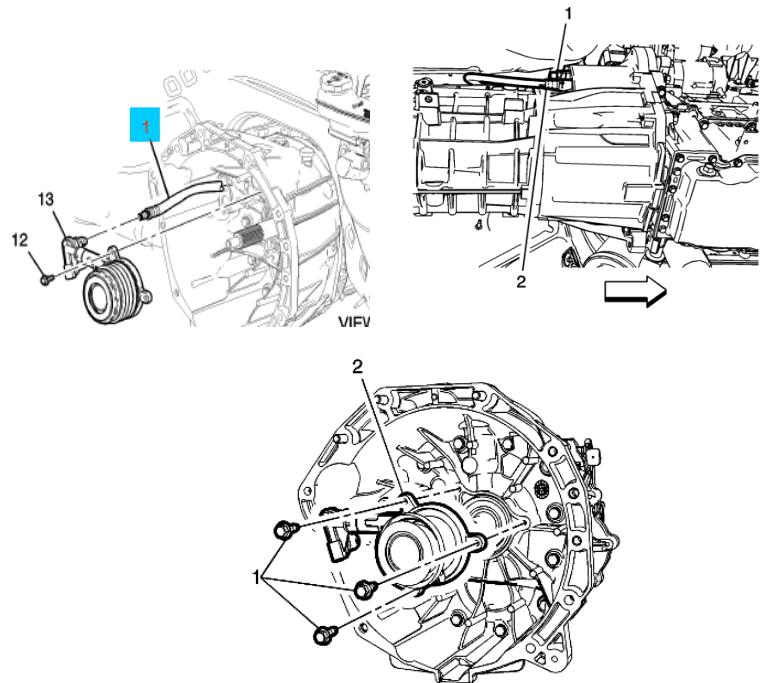
3. Prepare the transmission for attachment to the engine as follows
