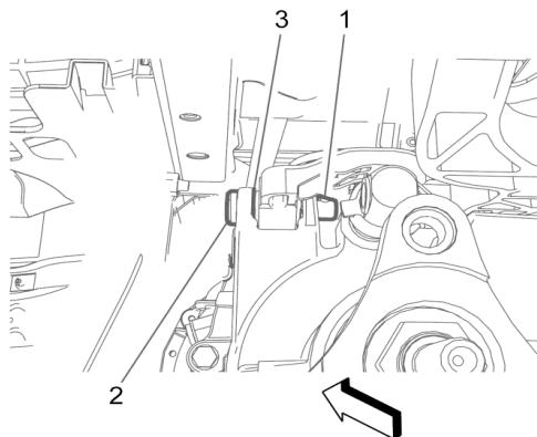
3. Install the left shift control assembly rod pin 24260856 (2).
