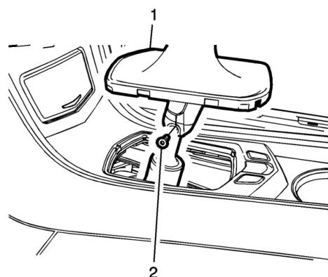
6. Install the shift control knob 24265701 using screw 11571034 torque to 7 NM (62 lb in) Thread locker should be used on this fastener. Note: The shifter boot is integral to the shift knob and it is up to the customer to integrate into the application. The illustration shows the console from the 2015 Cadillac ATS for reference.
