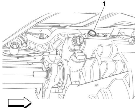
2. Install the right shift control assembly rod pin 24260856 (1).
