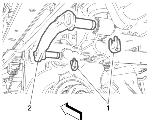
4. Install the shift linkage retaining clip 11087213 (1).
