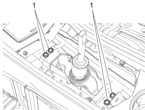
5. Four fasteners 11562426 are provided (1) securing the shift control assembly to body of the vehicle if customer desired. The illustration shows the production vehicle attachment to the transmission tunnel Bolt torque is **18 NM (13 lb ft)**
