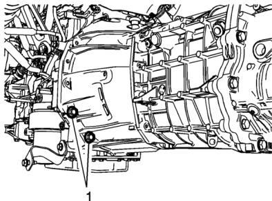
8. Install the upper transmission clutch housing to engine bolts and studs (1) and tighten to **50 NM (37 lb ft)**.
