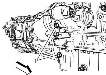
6. Install the two left lower transmission clutch housing to engine fasteners (1) and tighten to **50 NM (37 lb ft)**.
