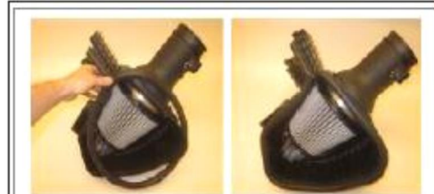
Figure 2: Installing hood seal and finished application
