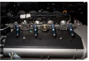
5. On the OEM fuel rail, locate the fuel pulse damper. Gently pry up on the tabs that hold it in place.
