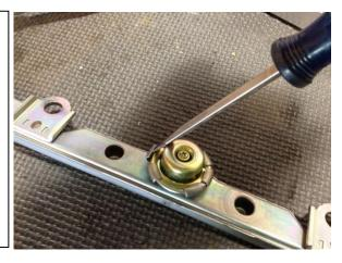
6. When all the tabs are bent out of the way, pull the pulse damper out by pulling straight out. Do not pull unevenly or pry from one side, as this may distort fuel pulse damper.
