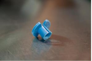
3. Insert the tool into the end of the fuel fitting. Make sure to surround the area with shop towels to absorb fuel contained in the pipe. While squeezing and applying pressure, pull the fitting away from the fuel pipe to release it from the fuel hose.
