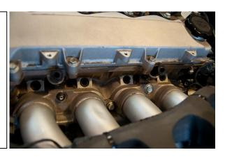
11. NOTE: If installing on a 2-Eleven or supercharged Exige-S with intercooler, some grinding is required of the intake manifold's aluminum boss as circled in the picture.
