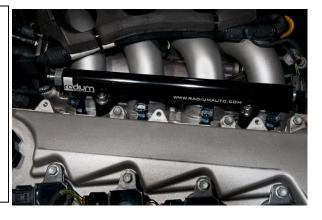
13. If installing 20-0012-00 or 20-0012-PK, the OEM fuel feed line will be reused. When tightening the hose to the fuel rail, hold the fuel rail fitting in place with a wrench. This avoids overstressing the fuel rail mounting tabs.
