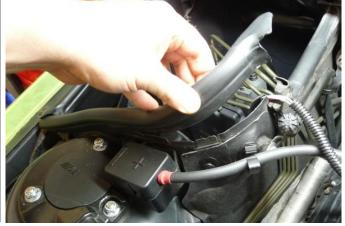
10. In order to pass the 2 hoses through the compartment wall, remove the factory plastic Phillips head fastener (shown) and plastic block off plate (shown).
