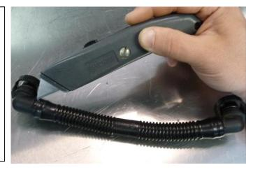
7. Cut a 19" section from included hose. Install between valve cover and catch can top port. If installing catch can back to intake manifold port, cut a 25" section from hose. Install between intake manifold and catch can side port.
