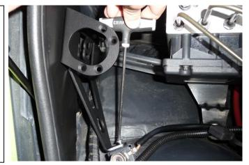
3. Lubricate the O-ring and screw the straight adapter fitting into the side (outlet) port. Install banjo fitting to the catch can top port.
