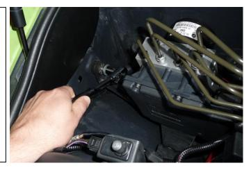
2. Install the mounting bracket to the 2 factory locations. For all models, use a 4mm Allen wrench and secure the included M6 button head bolt to the boss near the ground lug, as shown.
