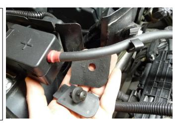
11. Slide the supplied clamps onto each hose and install the factory BMW plastic barb fittings. Lubrication may be required. To secure, use pliers and slide the clamps over each fitting. Press both OEM fittings back into place.
