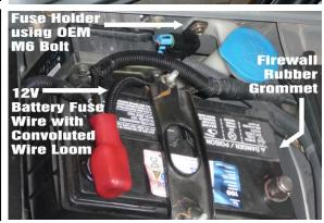
33. Use the convoluted wire loom for the trunk wiring, as shown. Reconnect the battery.
