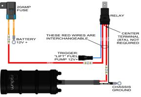
28. NOTE: After crimping both ring terminals in the schematic, give the wires a tug for verification. Use the included heat shrink and a heat gun to cover the 2 wire (relay and FST fuel pump) ground terminal connection to add strain relief to the crimp, as shown.
