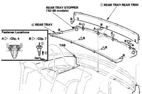
4. The rear trim can be removed from the interior but the rear tray MUST be removed from the trunk, as shown.
