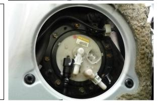
15. 2000-2005 S2000: The 2 short hoses and 2 long hoses will connect strategically to the FST. The short hoses connect to the OEM tubes previously disconnected from the fuel pump hanger. The long hoses will connect to the OEM fuel pump hanger.
