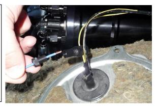
30. Insert the blue wire through the center section of the Posi-Tap connector. Screw the Posi-Tap connector together and give the wire a quick tug to make sure it seated properly.
