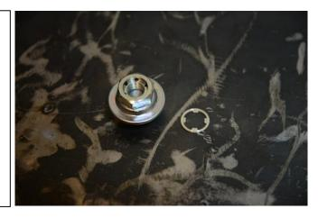
10. For 20-0111-PK or 20-0111-00 is used, install the fuel pulse damper adapter into the center port of the Radium fuel rail. **To prevent failure, the O-ring MUST be lubricated prior to assembly.**
