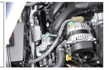
25. The black metal cover needs to be reused to provide mounting for the ECU. Modify it by cutting a large slot to clear the end fitting of the Radium fuel rail. This may take several test fitting iterations. CAUTION: Do not cut metal or create sparks near open fuel lines and gasoline.
