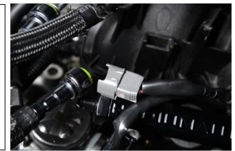
15. Orientate the #2 injector so that the electrical connector clears the OEM high pressure fuel pump.
