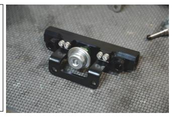
12. For 20-0111-00 or 20-0111-PK, install the included -6AN adapters into each end of the fuel rail, as shown. **To prevent failure, all O-rings MUST be lubricated prior to assembly.** Hold the fuel rail in a vice with non-marring jaws, and tighten the fittings with a 1" non-marring wrench.
