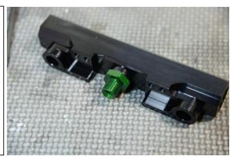
11. Place the crush washer from Step 9 on the adapter fitting then screw on the pulse damper. Tighten with a 7/8" or22mm wrench.
