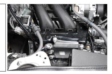
31. Turn the ignition to the ON position to allow the fuel pump to prime. Check for leaks. Start the engine; it may take longer than usual to start because air is being bled out of the system. Once started, check again for leaks. **Installation Complete**
