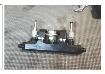
13. For some fuel rails purchased prior to October 2018, locate the electrical connector for the #2 (front) injector.
