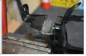
26. This picture shows the clearance slot around the end fitting of the fuel rail.
