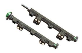
20. Inspect the lower grommets (shown) for debris and replace if needed. Verify that each injector port has a grommet.
