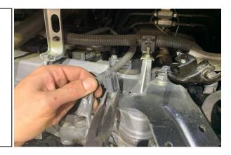
13. Unscrew the bolts and remove the brace shown from the rear of the engine (if equipped).
