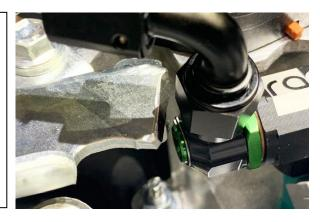
25. For those using the Radium Engineering plumbing kit, temporarily install the provided PushLok hose ends to the fuel rail end port fittings. Lineup the included hose and cut to length. Every application is different, but 5 inches (127mm) is typically best.
