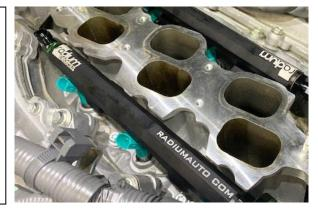
22. Fasten down the fuel rails using the included M8 bolts and washers and a 5mm Allen wrench.
