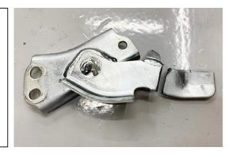
24. For those using the Radium Engineering plumbing kit, test fit the brace to make sure there is enough clearance with the crossover hose fittings. Once verified, reinstall the braces (if equipped).
