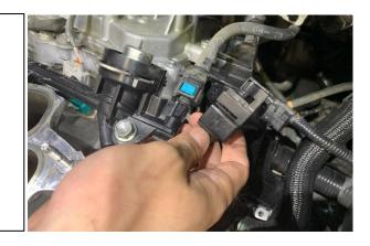
15. Squeeze the blue SAE quick connect locks and simultaneously pull the fuel feed line off the fuel rail. Be prepared with rags as fuel will leak out.
