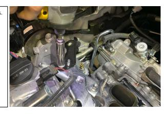
12. On the opposite side of the engine, pull the electrical stay up off the stud shown.
