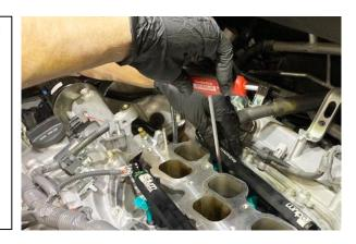
23. For Toyota 2GR-FE engines which use the additional engine braces, modify the brace (shown) with a cut-off wheel in the area illustrated.
