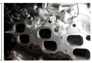
21. To prevent failure, lubricate the injector O-rings with a petroleum-based oil. Install the fuel injectors previously removed from the factory rails into the Radium Engineering fuel rails. Be very careful not to damage the O-rings.
