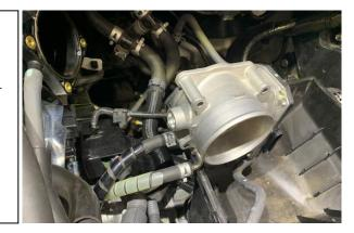
6. Locate the 5/8" crankcase breather hose just downstream of the throttle body (d). Using a pair of pliers, squeeze the spring clamp and slide it down the breather hose a few inches. Now, pull this hose off the intake manifold plenum.
