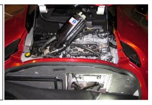
10. It is advised to plug (or tape over) all 6 cylinder intake ports to prevent objects from falling down into the engine.
