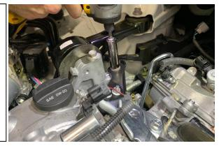
11. Using a 12mm socket wrench, remove the 2 nuts and 1 bolt from the two braces. Remove the black and silver braces from the engine.
