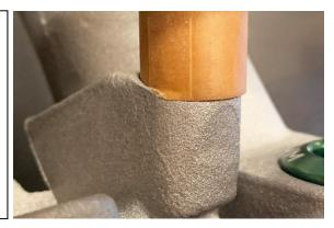
7. As a test, push the fuel injectors downward until they bottom out. Now inspect the injectors' upper O-rings and confirm they are still inserted into the fuel rail injector bores. Do not pressurize the fuel system until the proper height is achieved.
