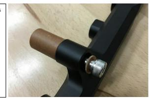
6. Place the fuel rail on the lower intake manifold. If using the OEM Nissan RB25DET manifold, there is a chance the insulating spacers may create a slight interference. This is normal and the severity will depend on the machining in the casting. As shown, grinding is typically not necessary. NOTE: This will not be the case with aftermarket intake manifolds.
