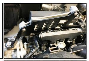
6. The direct injection ECU is chassis grounded through the engine using the bottom OEM mounting bolt. If this connection is forgot, the engine will not run. Secure with a 10mm socket wrench.
