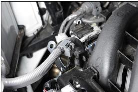
3. Remove the three M6 bolts holding the direct injection ECU to the OEM brackets using a 10mm socket wrench.
