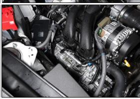
4. Set the new Radium bracket in place. Using a 12mm socket wrench, secure using the two OEM M8 bolts.
