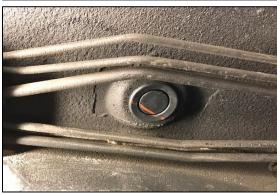
9. Lineup the filter bracket assembly to the open threaded holes. Install the 3 provided button head bolts to the chassis. If necessary, pull and spread the OEM hard lines to permit additional space.
