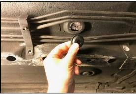
8. Flip the plug around and reinsert until it locks in place, as shown. This will provide additional room for the fuel filter assembly.
