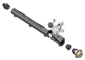
4. For ease of installation, apply a light coat of oil to the injector O-rings, intake manifold injector seats, and fuel rail injector bores. Fully insert the injectors into the fuel rail bores, as shown.
